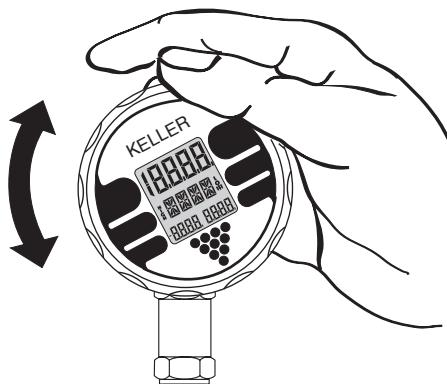
The splash-proof cover of the *Intelligent Manometer* is sealed with an O-ring and may easily be removed by hand by turning the display ring beyond the limit stop (see "Battery Change" in Chapter "Notes" on page 12).
