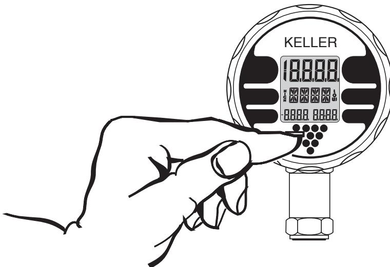
The *Mano-Mode* is the standard mode of the *Intelligent Manometer*. Since the function of secondary displays can be selected (see *Dise-Mode*), the individual segments are described with the peak- and trough pressure display:
