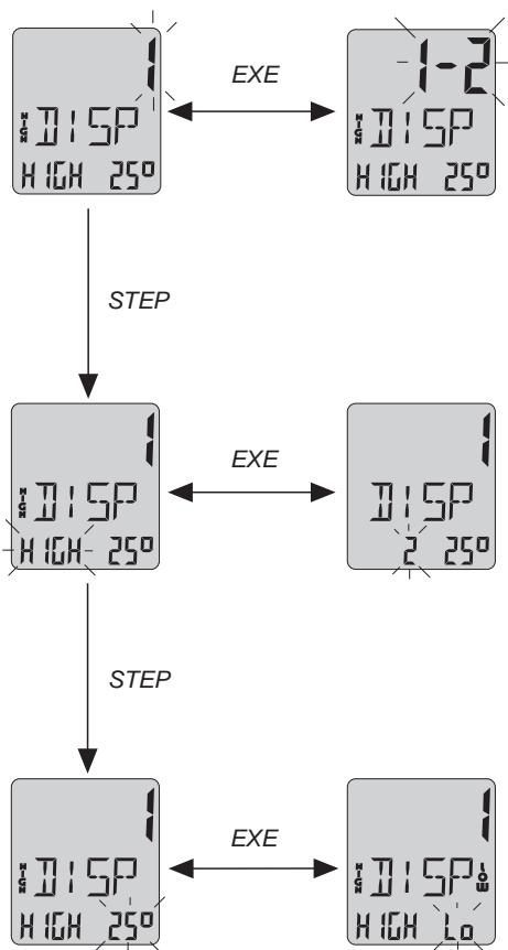
After activating *DISE*, the instrument displays the actual settings. The display that is now flashing can be changed by activating *EXE*.
