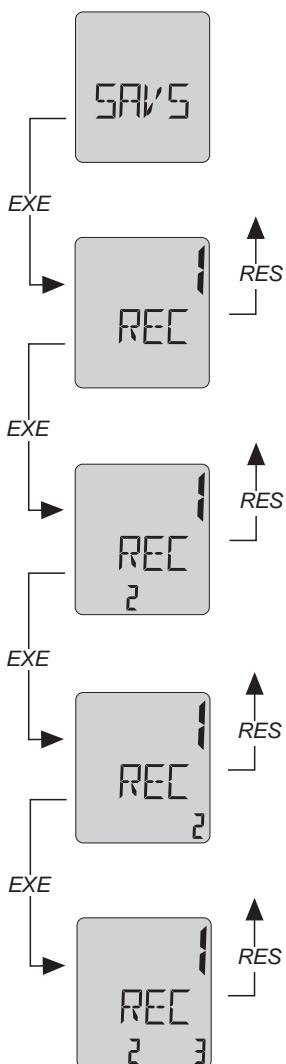
The settings programmed in *DISE*, which are now active, can be selected for storage under SAVS. Only the variables which are selected under SAVS will later actually be stored in the *Record-Mode*.
